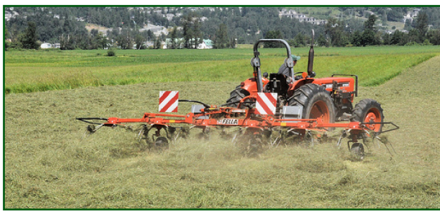
Figure 6. Tedder used for inverting dried forage to speed drying. Photo by permission of Pat Meyer.
